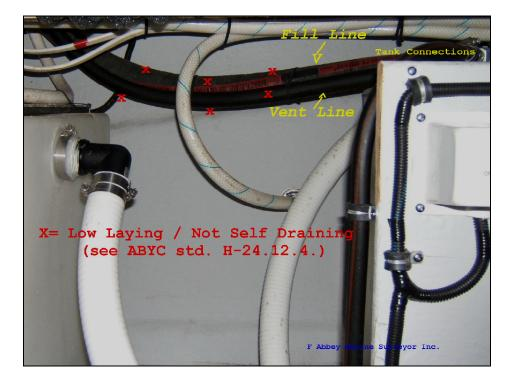
The photograph (of the port fuel tank) shows that the run, of the fill and vent lines rigged to each of the two (installed port & stbd. in the engine space) fuel tanks, are not self-draining. This situation does not comply with the provisions of **A.B.Y.C Standard H-24.12.4** "Fuel fill lines shall be self-draining and run as directly as practicable from the deck plate to the fuel tank connection and **H-24.13.7** "Tank vent systems shall be self-draining".
